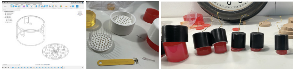
Fig. 4. The design, printing, and assembling process of light spots used for data projections
