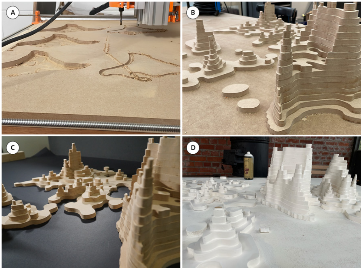
Fig. 3. The four images show the individual stages of the elevation map creation. a) CNC cutting the wood shapes, b) spatial construction of the individual layers c) surface optimization d) surface coating, 2023.
