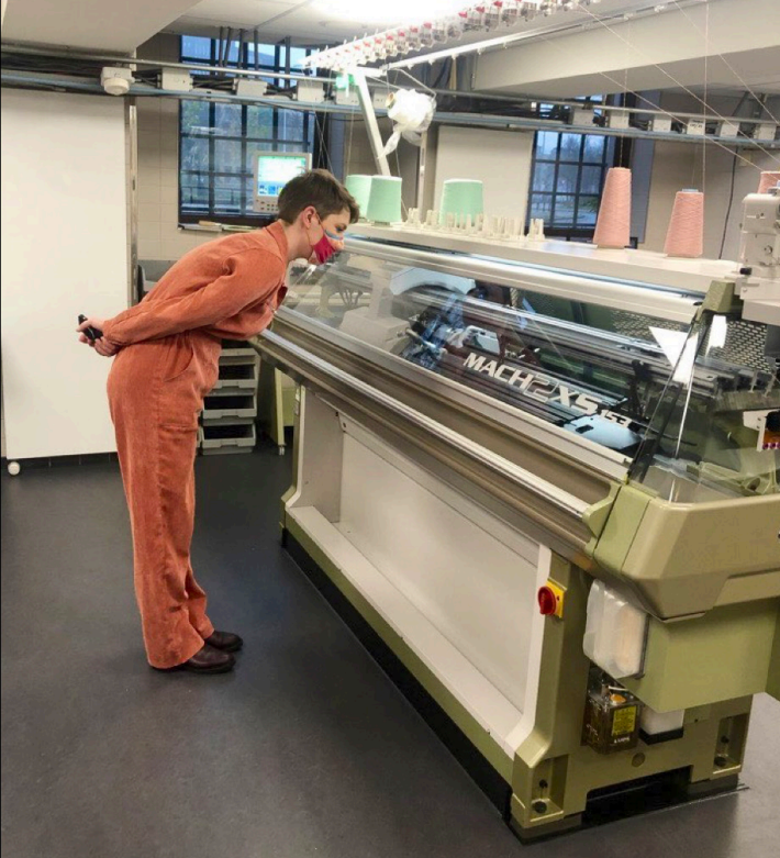
Figure 3. Knitting the sweater on our Shima Seiki Mach 2XS knitting robot.
